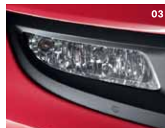
03 Static cornering function for front fog lights.
